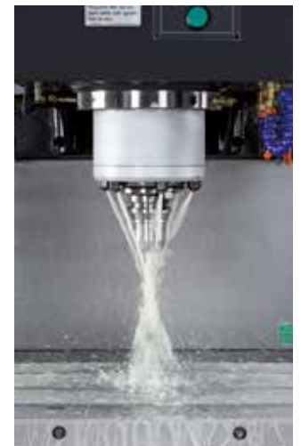
▲ Spindle Ring Sprinkler
