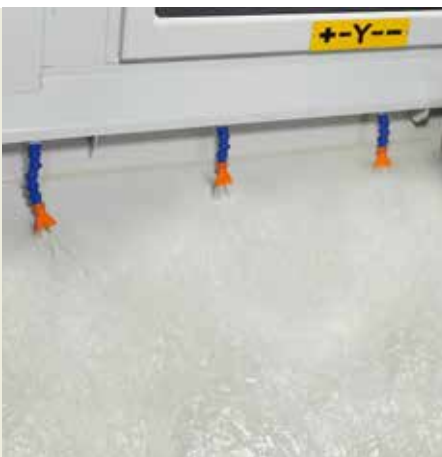
▲ Chassis Chip Flushing
